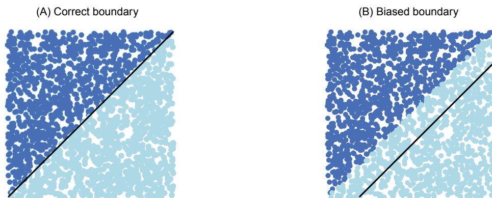
Figure 8.2: Thresholds dictate the placement of decision boundaries, which in turn influence the classification error.
